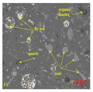
particle length, width) and reflectance fingerprint of each individual particle. Based on the reflectance fingerprint, the particle can be classified as a coal or non-coal particle, allowing CSIRO to count the number of coal particles and estimate the mass of coal particles in each size range.
