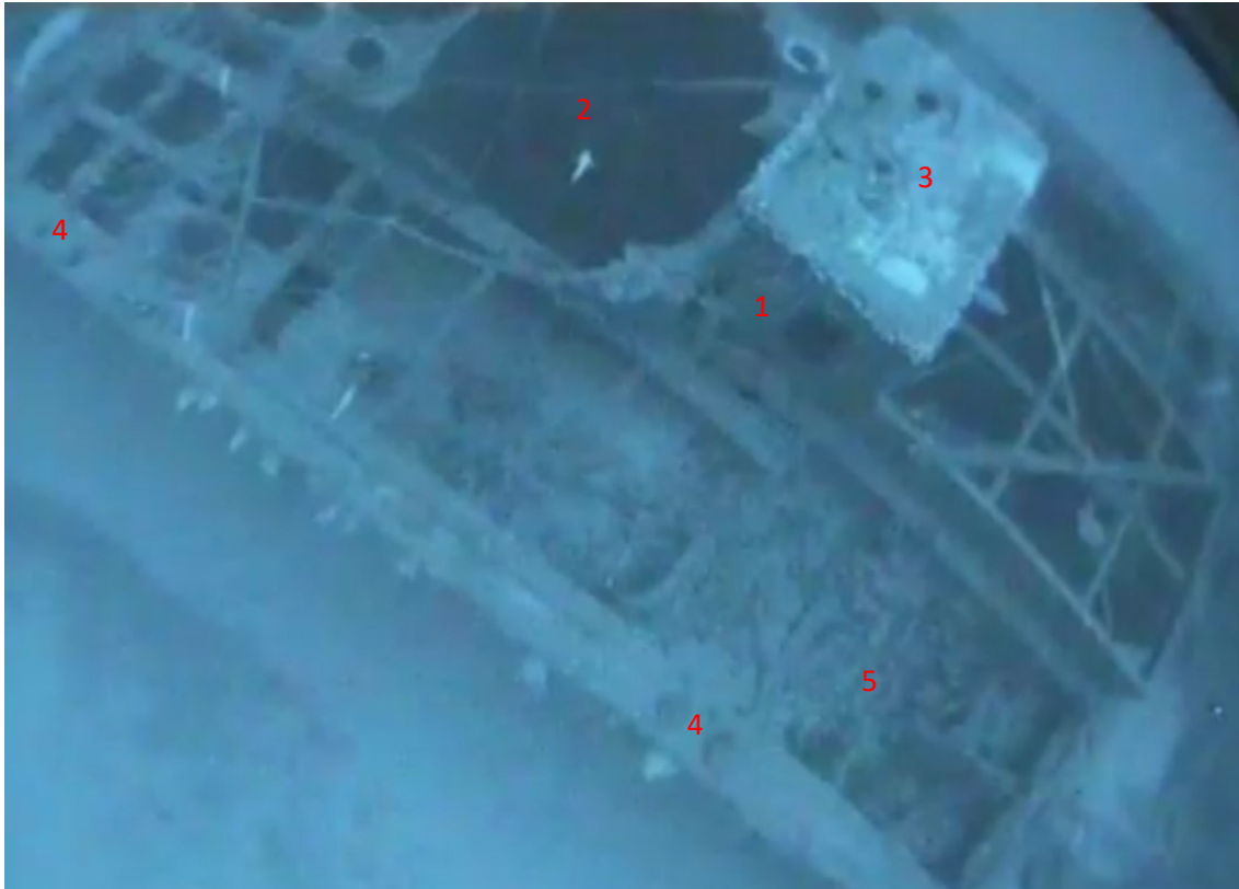
Figure 76: Deckhouse structure (1) abaft the funnel (2). Note the outlets in the roof, probably indicative of ventilation or chimney/ exhaust outlets (3) bitts on port main deck (4); and coal in the coal bunkers under the main deck (5) (Image: CSIRO 2023 - 2715)
