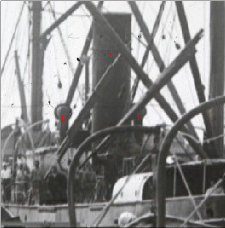
Figure 113: Nemesis loading Timber in WA showing the location of the funnel and two stokehold ventilator tubes (Image: SLWA n.d., (R4c) - Nemesis Loading Timber in WA)
