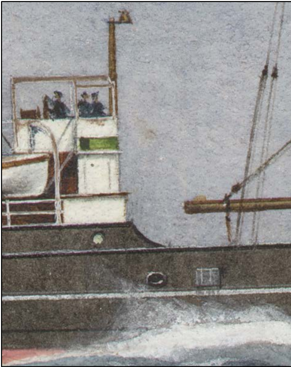
Figure 116: Main sheerstrake plating on the hull of the Nemesis (Image: Green c 1900 Nemesis (# wp004986))
