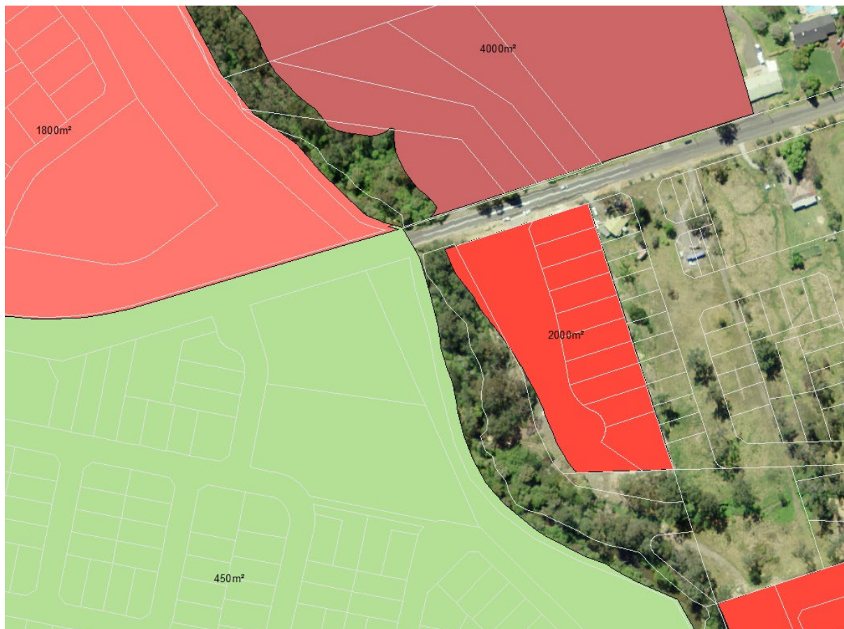
Figure 1 Example of an LEP lot size map specifying different minimum lot sizes over part of the land within the LEP
