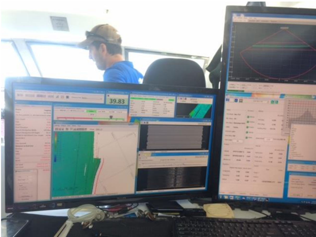
Figure 3.2 Onboard setup of Hypack, POSView and R2Sonic interface. Photo: T Ingleton/OEH
