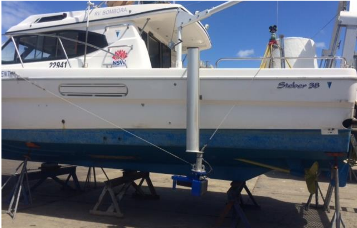
Figure 2.4 RV Bombora hardstand survey March 2018 – R2Sonic 2022 single-head locked into position with fore and aft stops. Photo: T Ingleton/OEH
