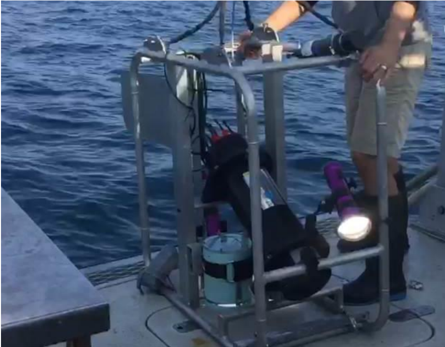
Figure 4.6 OEH towed video setup with forward looking (30°) video camera providing real-time video feed via fibreoptic cable to the surface and downward looking still cameras with laser pointers for scale. Photo: J Miller/OEH
