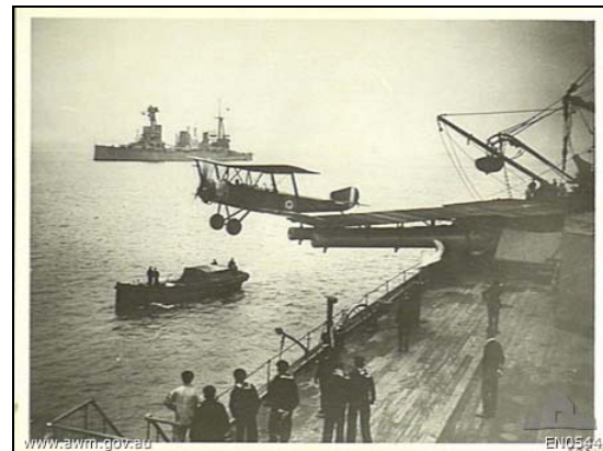
Members of the ships company watch as a two seater Sopwith 1 ½ strutter biplane takes off from the ships starboard gun turret (Photo: Australian War Memorial image # EN0544)
