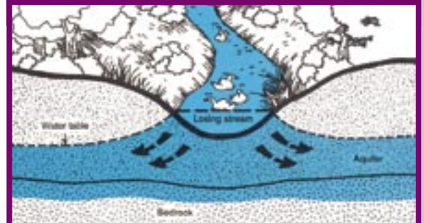
Fig 13. Groundwater. Gaining streams and losing streams (Reference 8)
