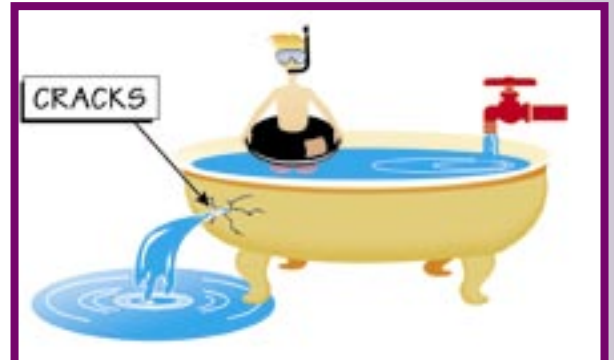
Fig 22. Problems with secondary porosity in an essentially impermeable cast iron bath tub
