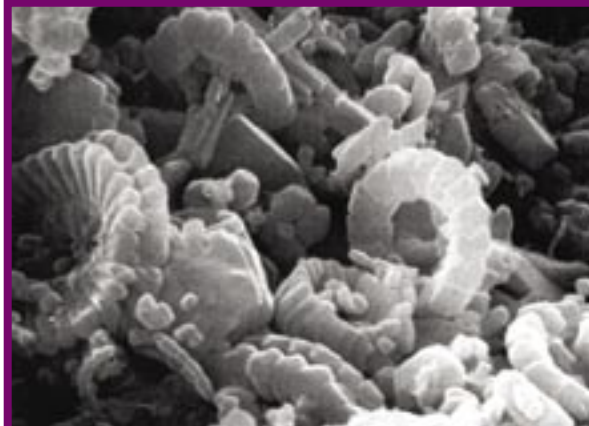
Fig 16. Electron photomicrograph of a low permeability rock formed by shells of micro-organisms. Although the rock's porosity is high - 46%, its pores are very small
