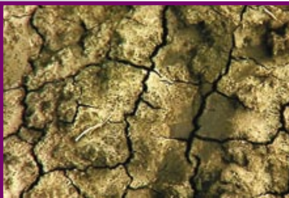
Fig 23. Desiccation cracks in clay (Reference 24)
