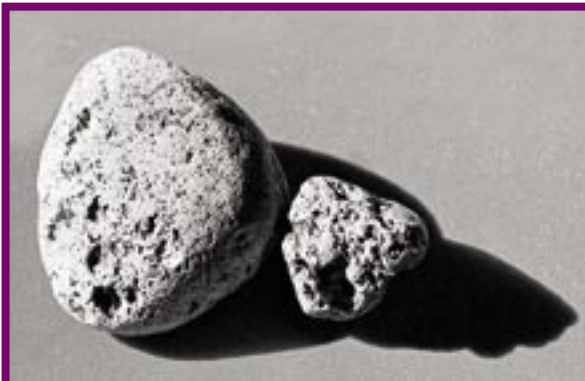
Fig 24. Pumice: a very porous material, but also very impermeable due to the lack of interconnections between its voids
